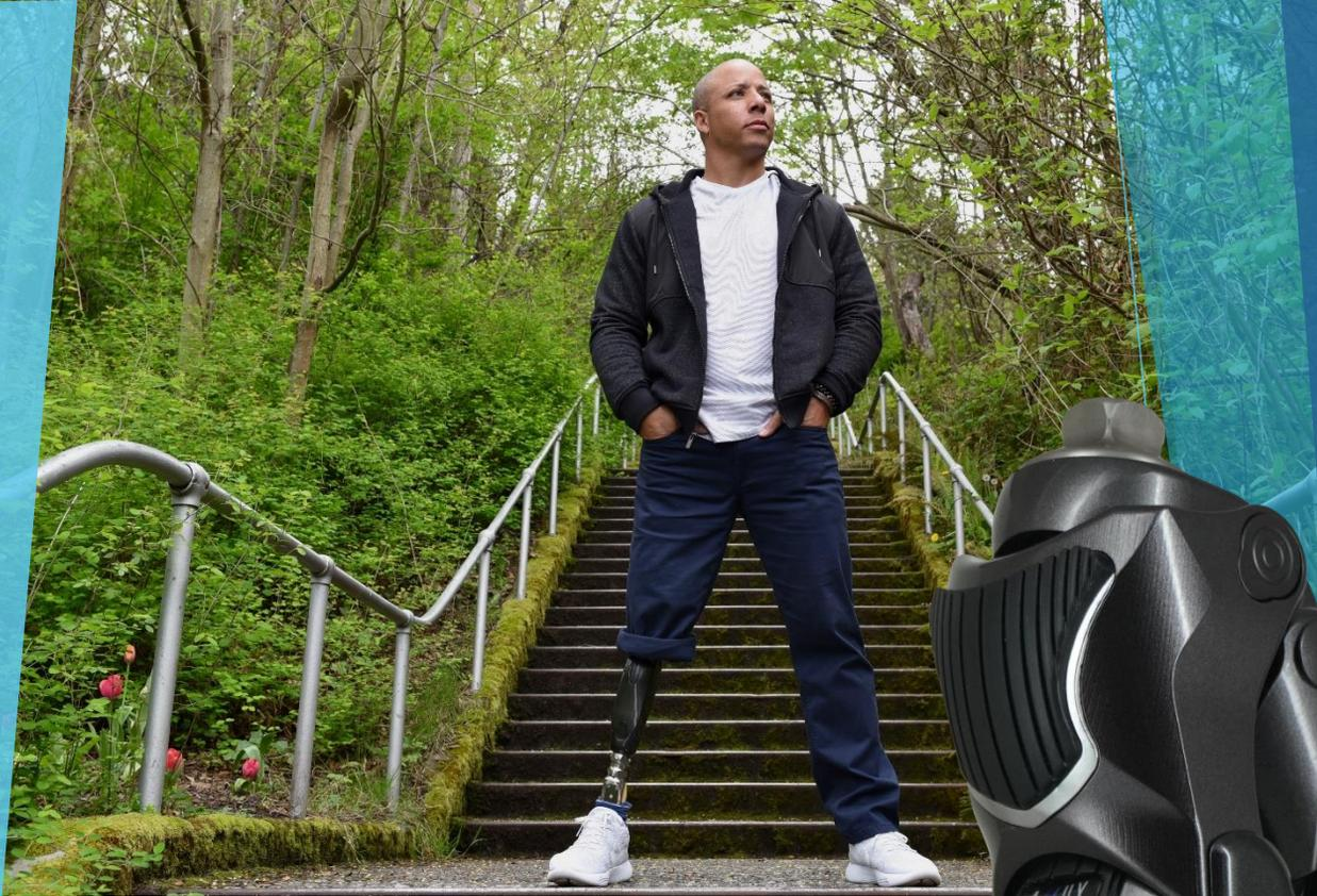
4-Bar Hydraulic Microprocessor Controlled Knee
